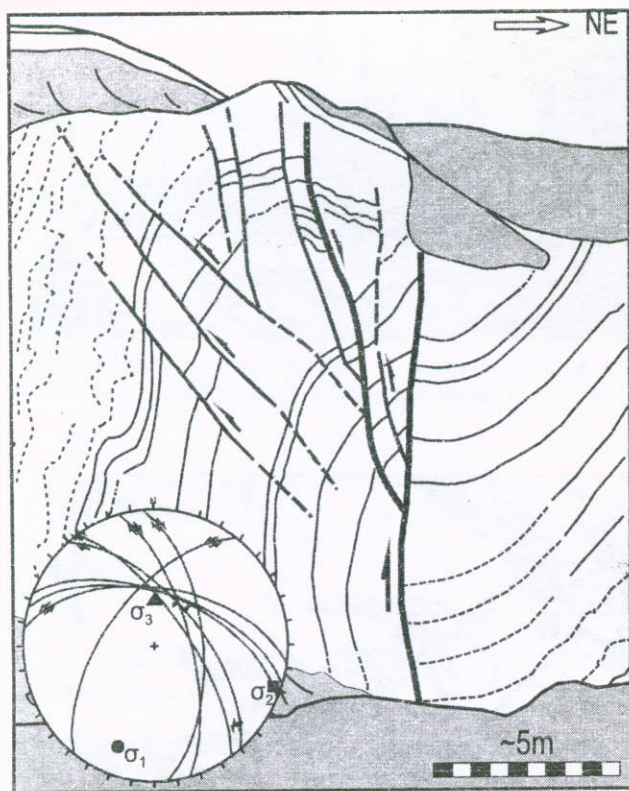
Figure 3: Interpretation of an outcrop in NW of the village of Gugark showing the complexity of the fault near the surface. Stress tensor obtained from population of micro-faults near the village shown below.
